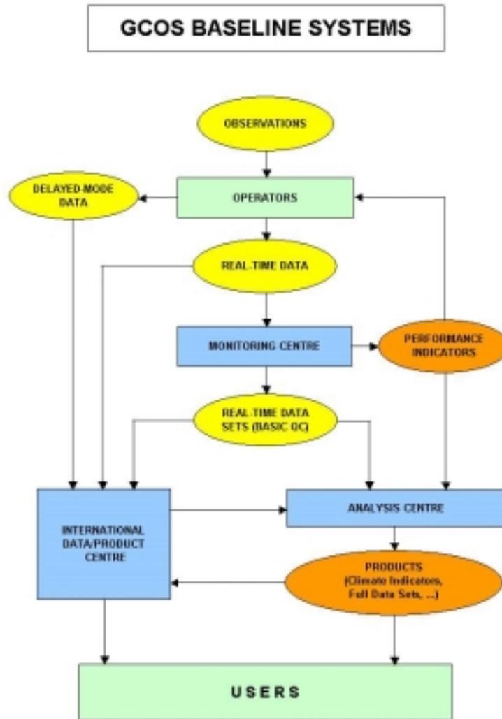
Figure 2. Schematic of the components of a typical GCOS baseline network.
